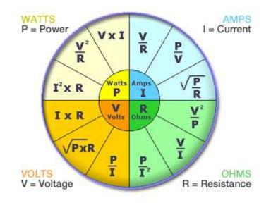
Using This Chart You Can Easily Calculate The Wattage, Current (Amps), Ohms, and Voltage For A Device!
